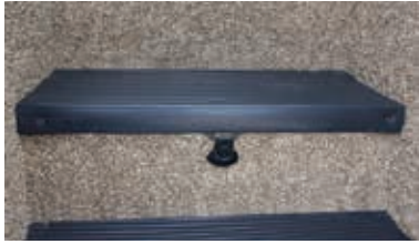
Typical Class C motorhome auxiliary battery location (under entrance step)
