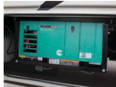
Typical motorhome generator
