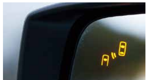
Illustration of mirror with blind-spot indicator (actual indicators and symbols may vary from this illustration)
