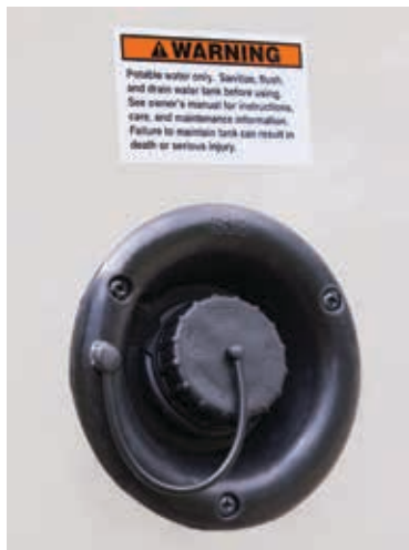
Typical fresh water gravity fill
