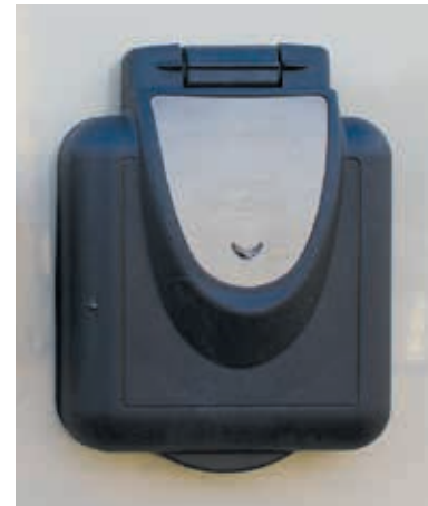
Typical shore line power cord connection port
