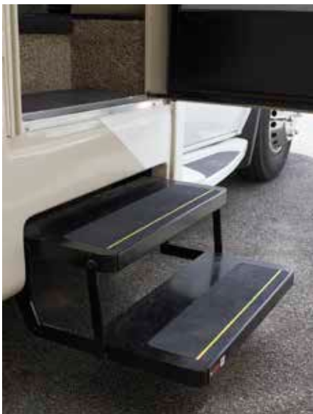
Typical powered entry step. Depending upon motorhome model, steps may have one or more treads.
