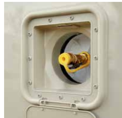
Typical external propane hook-up
