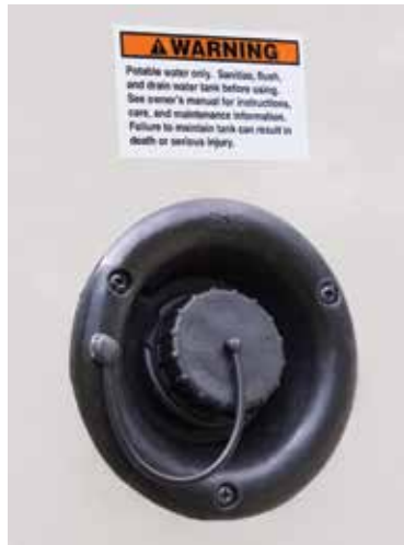
Typical fresh water gravity fill
