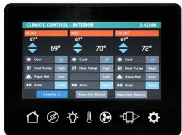
Typical multiplex control panels depicting climate control display
