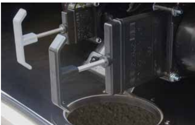
Typical termination valve configuration
