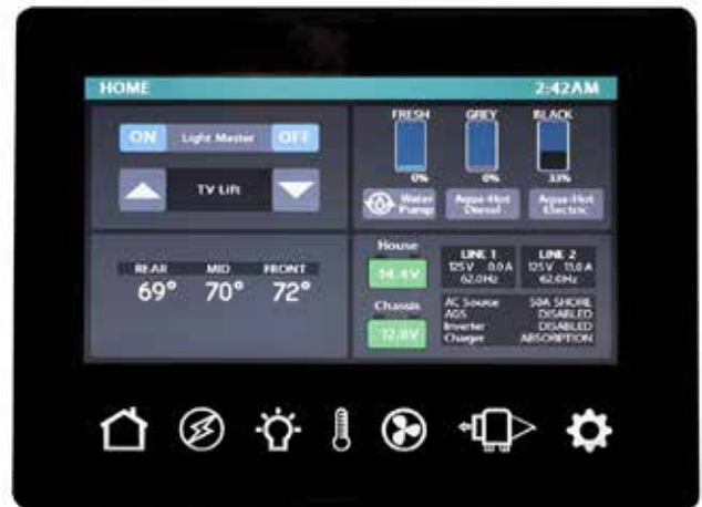
Typical multiplex main control panel. Electrical system monitoring is usually located on the main menu (House) screen.
