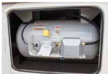
Typical propane gas tank
