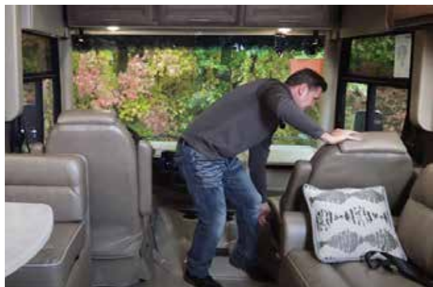
Figure 2. Recline both front seat backs before lowering the powered over-cab bunk.
