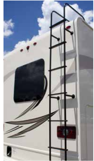
Typical roof ladder
