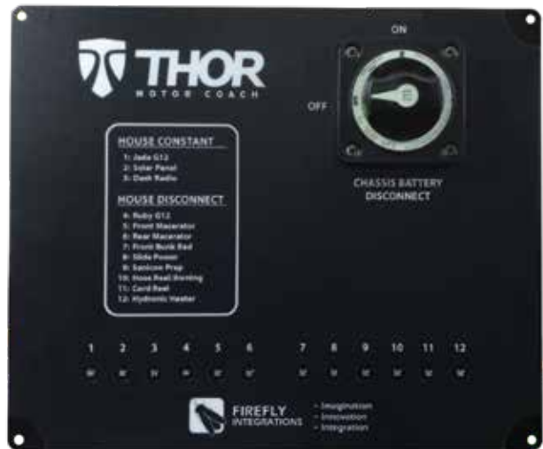
On select diesel motorhomes, the master battery disconnect switch, along with 12 volt circuit breakers, is located on a panel installed in a service bay of the motorhome.
