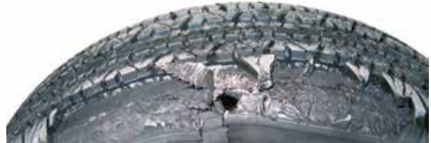
Tire pressure under and/or over inflation can cause serious tire failure
