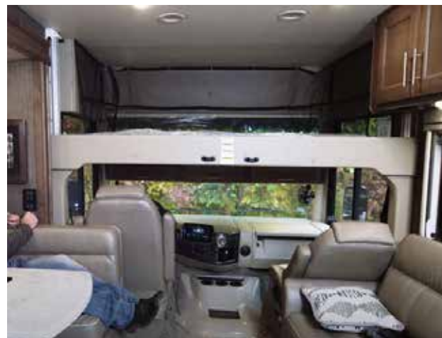
(Above) Powered Over-cab Bunk in the Raised position. (Below) Powered Over-cab Bunk in the lowered position. Your dealer is can instruct you in the operation of beds, bunks, and convertible furniture.
