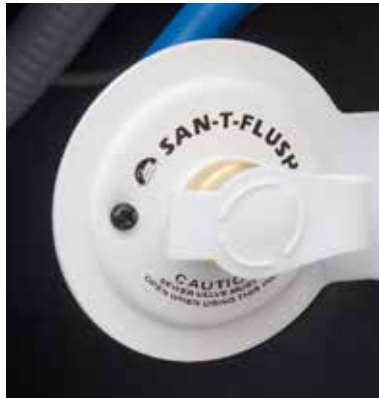
Typical black tank flush
