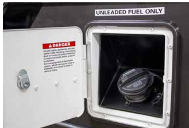
Fuel Tank Inlet for Fuel Transfer System
