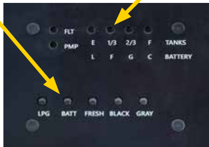
Typical multiplex main control panel. Electrical system monitoring is usually located on the main menu (House) screen.
