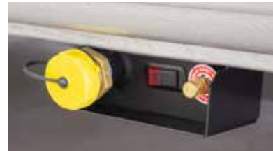
Propane access panel, positioned along the lower left side of the vehicle
