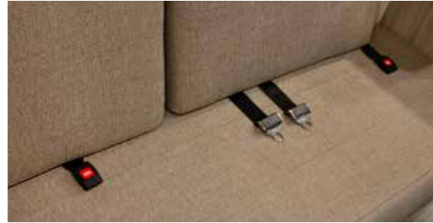
Typical passenger seat belts located in a dinette or sofa seating area
