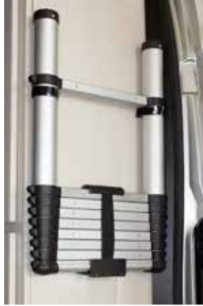
Collapsible ladder stowed behind rear door. The magnetic ladder bracket is stowed on the inside of the left-side rear door.
