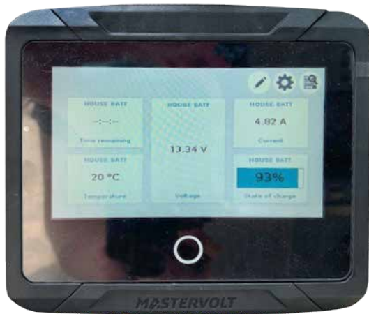
Illustration of Mastervolt control panel in the battery monitor mode
