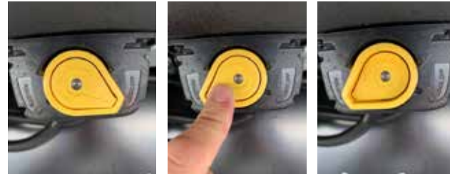
Safety Relays in the OFF position
