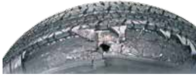
Tire pressure under and/or over inflation can cause serious tire failure
