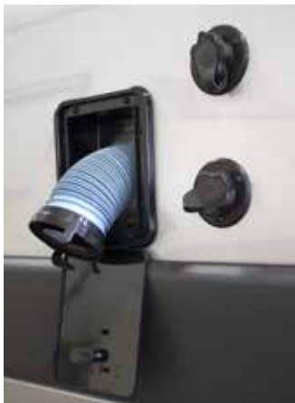
City water fill connection, along with a storage chamber for the sewer hose. This image for reference only. The water ports on Class B motorhomes vary in type and location due to floor plans and features.
