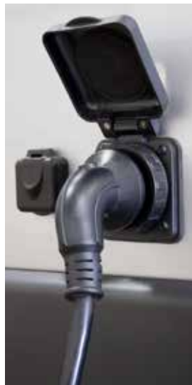
Typical shore line power cord connection port
