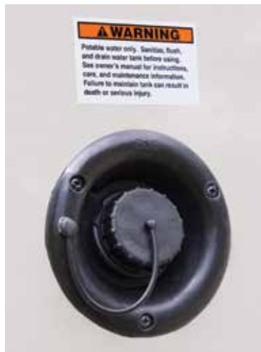
Typical fresh water gravity fill
