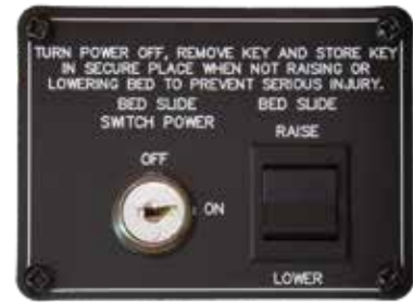
Typical keyed bed lift safety switch
