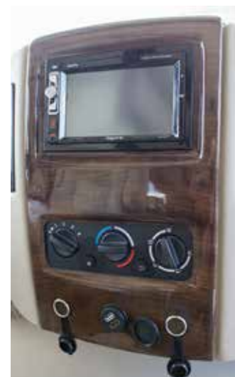
Typical Class A heating and air conditioning dash controls
