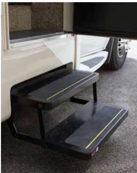
Typical powered entry step. Depending upon motorhome model, steps may have one or more treads.
