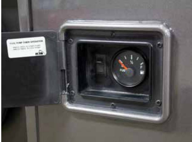
Fuel Pump Switch and Fuel Gauge for Fuel Transfer System
