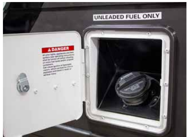
Fuel Tank Inlet for Fuel Transfer System
