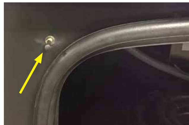
Fuel Pump Safety Lock-out Switch
