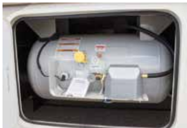
Typical propane gas tank
