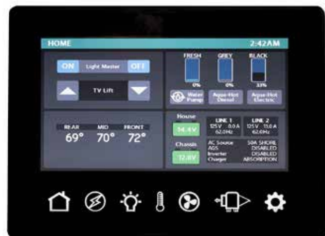
Typical multiplex main control panel. Features vary depending upon model and floor plan
