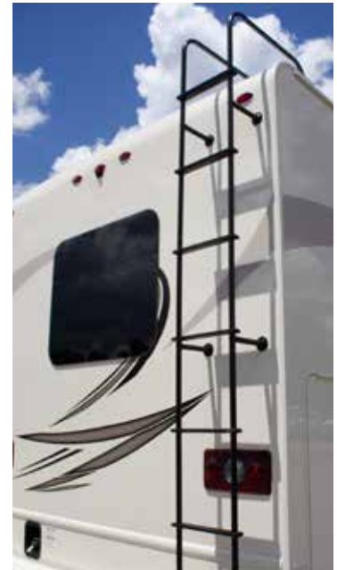
Typical roof ladder
