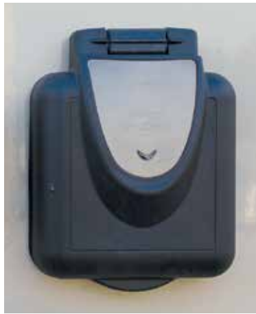
Typical shore line power cord connection port
