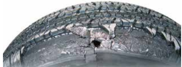
Tire pressure under and/or over inflation can cause serious tire failure
