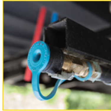
Exterior LP Connection
